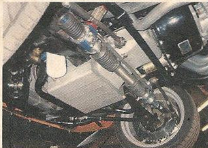
Thorough wash downs and maintenance after each rally keeps the Boss looking as good as its first day out of the shop. A Total Control power rack handles steering duties, while the Roush oil pan nicely controls 7 quarts of oil. Note the additional crossmember behind the rack.
