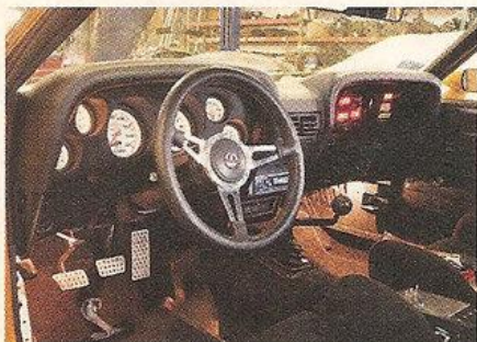
A JME gauge panel fills the left side of the dash while a custom clock panel with Brantz rally timers occupies the right side.
