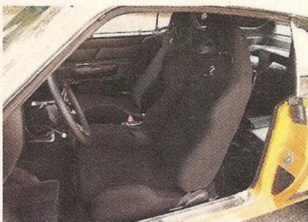
Corbeau rally seats provide the much needed lateral support for rally events.
